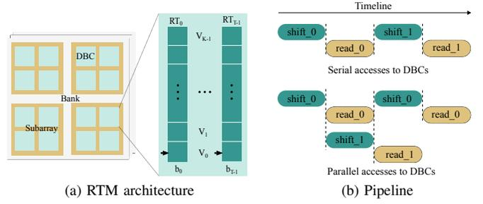
Figure 2. An overview of the RTM architecture. A DBC consists of  $T$  (e.g., 32) nanowires and stores  $K$  (e.g., 64)  $T$ -bit words in a bit-interleaved fashion. The figure on the right shows parallel accesses to DBCs for improved bandwidth utilization and hiding shift latency.
