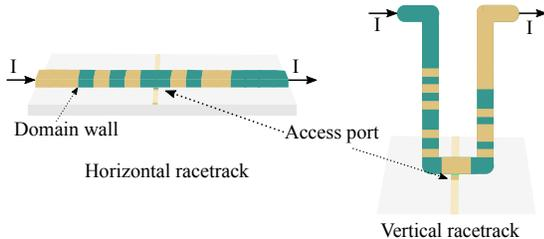
Figure 1. RTM cell structure
